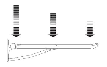
All tests have been conducted by mounting the products on a solid wall. This is what Pressalit recommends. The lifespan of the product is not affected by the wall type. However, the overall solution will inevitably be influenced by the condition and material of the wall. Therefore, reinforcement should always be used if the wall is not stable.
