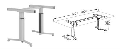
Electric lift for freestanding worktop. For worktops from 1400 - 2000 mm. Height adjustable 300 mm. Including 2 telescopic legs, longitudinal and cross braces and switch.
