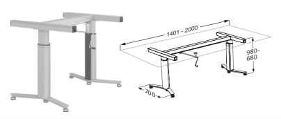
Manual lift for freestanding worktop. For worktops from 1400 - 2000 mm. Height adjustable 300 mm. Including 2 telescopic legs, longitudinal and cross braces and crank handle.
