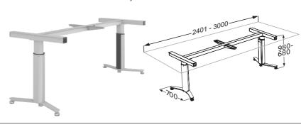
Electric lift for freestanding worktop. For worktops from 2401 - 3000 mm. Height adjustable 300 mm. Including 2 telescopic legs, brackets, longitudinal and cross bracesand switch.
