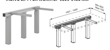
INDIVO lift for worktop, with three motors and control box. Incl. cross brace and two brackets. Height adjustable up to 300 mm with switch or wired remote control. For worktop length 1001-1400 mm.
