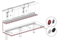
Interconnection of safety RK1374 For interconnection of: - Safety bars for worktop - One safety plate for wall cupboards.
