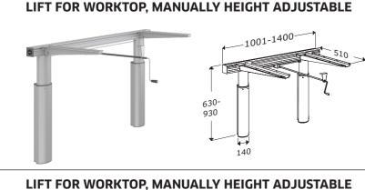
Manual lift for worktop. Lift for worktop, with a crank handle Including 2 brackets Lengths from 1001-1400 mm. Height adjustable 300 mm.
