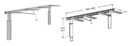
Manual lift for worktop. Lift for worktop, with a crank handle Including 4 brackets Lengths from 2001-2400 mm. Height adjustable 300 mm.
