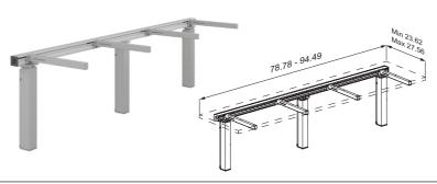
INDIVO lift for countertop, with three motors and control box. Max. load: 330 lbs/150 kg including the countertop. Incl. cross brace and four brackets.
