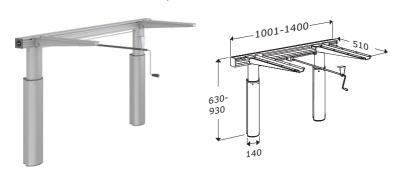
Manual lift for countertop. Lift for countertop, with a crank handle. Including 2 brackets. Lengths from 39.4"-55.1"/1001-1400 mm. Height adjustable 11.8"/300 mm.
