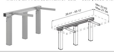
INDIVO lift for countertop, with three motors and control box. Max. load: 330 lbs/150 kg including the countertop. Incl. cross brace and two brackets.
