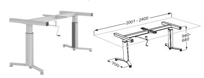
Manual lift for freestanding countertop. For countertops from 78.8" - 94.5"/2001 - 2400 mm. Height adjustable 11.8"/300 mm. Including 2 telescopic legs, brackets, longitudinal and cross braces and crank handle.
