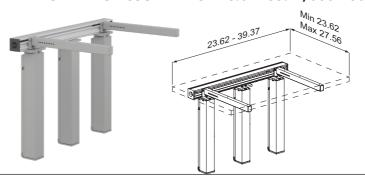
INDIVO lift for countertop, with three motors and control box. Max. load: 330 lbs/150 kg including the countertop. Incl. cross brace and two brackets.
