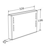
Extension fitting, 15.7"-47.2"/400-1200 mm, 1 pc. For installing cabinets higher than 27.7"/704 mm.
