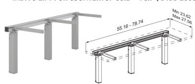
INDIVO lift for countertop, with three motors and control box. Max. load: 330 lbs/150 kg including the countertop. Incl. cross brace and three brackets.
