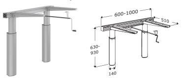
Manual lift for countertop. Lift for countertop, with a crank handle. Including 2 brackets. Lengths from 23.6"-39.4"/600-1000 mm. Height adjustable 11.8"/300 mm.
