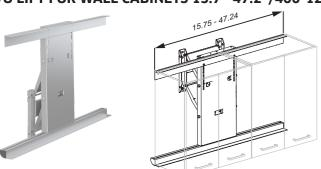
INDIVO lift for wall cupboards, with one motor and control box. Max. load: 240 lbs/110 kg including the cabinet. Height adjustable 16.9"/430 mm with switches or wired remote control. When height adjusting downward, the lift will also move 7.1"/180 mm towards the user. For wall cabinets width 15.7"-47.2"/400-1200 mm.
