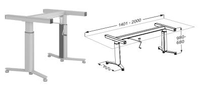
Manual lift for freestanding countertop. For countertops from  $55.1^{\circ}$  -  $78.7^{\circ}$ /1400 - 2000 mm. Height adjustable  $11.8^{\circ}$ /300 mm. Including 2 telescopic legs, longitudinal and cross braces and crank handle.
